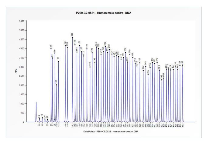
**Figure 1**. Capillary electrophoresis pattern from a sample of approximately 50 ng human male control DNA analysed with SALSA MLPA Probemix P209 Glycine Encephalopathy (C2-0521).
