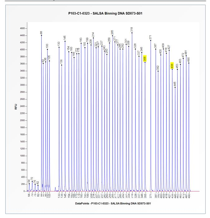
**Figure 2**. Capillary electrophoresis pattern from SALSA Binning DNA SD073-S01 (approximately 50 ng) analysed with SALSA MLPA Probemix P103 DPYD (C1-0323). The location of the c.1129-5923C>G mutation-specific probe at 355 nt and c.1905+1G>A mutation-specific probe at 436 nt are indicated.
