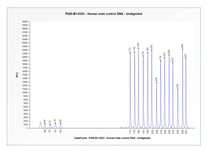
**Figure 1**. Capillary electrophoresis pattern from a sample of approximately 50 ng <u>undigested</u> human male control DNA analysed with SALSA MLPA Probemix P200 Reference-1 (B1-0323), for the quantification of copy numbers.
