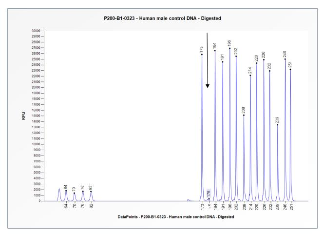
**Figure 2**. Capillary electrophoresis pattern from a sample of approximately 50 ng <u>digested</u> human male control DNA analysed with SALSA MLPA Probemix P200 Reference-1 (B1-0323), to determine the methylation status. The location of the digestion control probe is indicated by an arrow.
